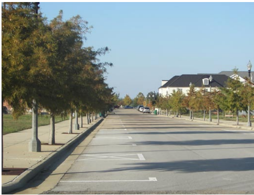
Figure 12.2 Continuous pedestrian thoroughfares like this sidewalk promote safe pedestrian use. Street trees help to buffer the pedestrian area from the street.
