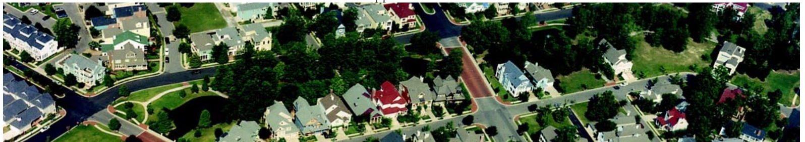
Figure 19.2 This residential neighborhood preserved a sensitive site area with existing mature trees and used the area for buffering the site and as a pedestrian area, equipped with walking trails.
